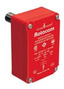
The Rotacam is available with two N.C. safety contacts and one N.O. auxiliary contact. The switch includes the necessary safety-related functions, such as forced-guided contacts and a tamper-resistant mechanism, allowing machinery to be safeguarded in compliance with the machinery directive.
